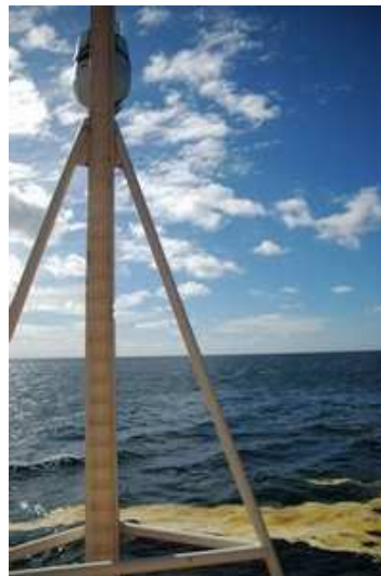
SensorPack mounted in the front mast with oil in front of the vessel
