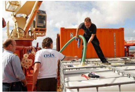
Oil sucked from the oil tanks
